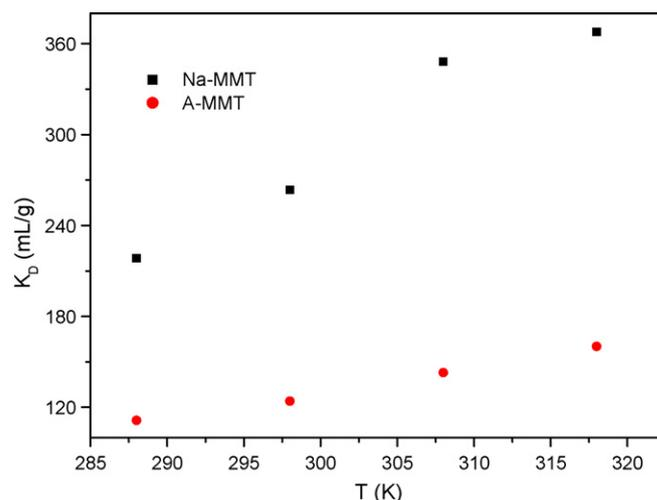
**Fig. 8.** Plot of distribution coefficient  $K_D$  against temperature for adsorption of Ni<sup>2+</sup> onto Na-MMT and A-MMT (Ni<sup>2+</sup> concentration, 100 mg/L; adsorbent dose, 6 g/L; pH, 6.5 ± 0.1; reaction time, 300 min; temperature 25 ± 0.1 °C; 200 rpm).
