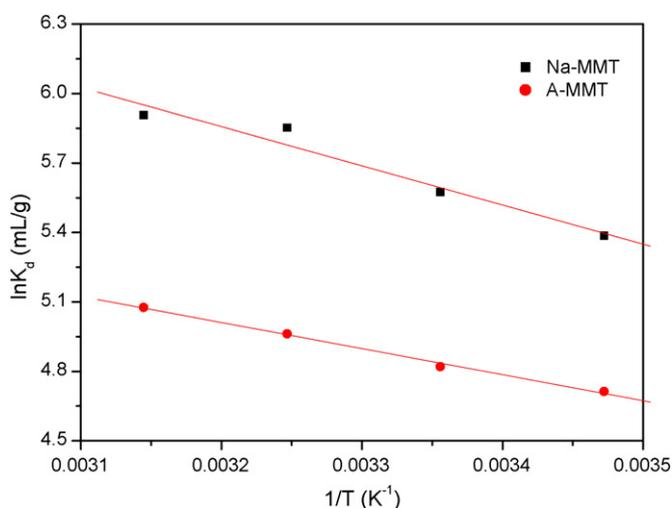
**Fig. 9.** Plots of  $\ln K_{(D)}$  vs.  $1/T$  for Ni<sup>2+</sup> adsorption onto Na-MMT and A-MMT (Ni<sup>2+</sup> concentration, 100 mg/L; adsorbent dose, 6 g/L; pH,  $6.5 \pm 0.1$ ; reaction time, 300 min; temperature  $25 \pm 0.1$  °C; 200 rpm).
