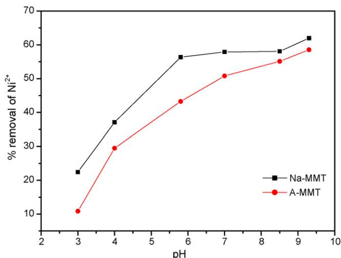
**Fig. 4.** Effect of pH on Ni<sup>2+</sup> adsorption (Ni<sup>2+</sup> concentration, 100 mg/L; adsorbent dose, 6 g/L; equilibrium time, 300 min; temperature 25 ± 0.1 °C; 200 rpm).
