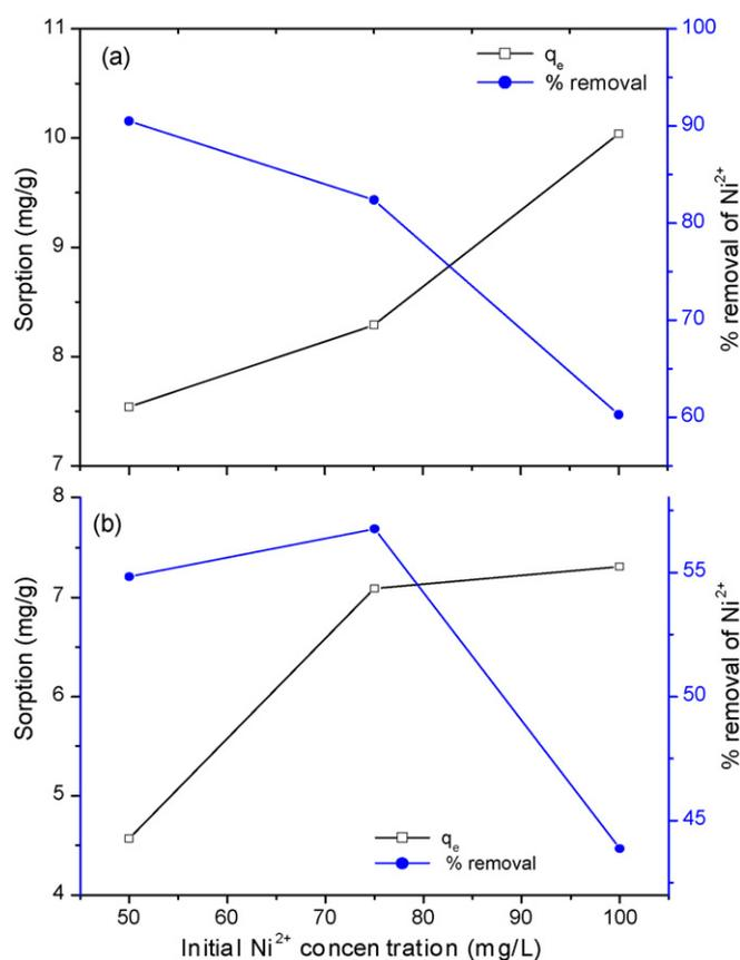
Fig. 5. Effect of initial concentration on adsorption of  $\text{Ni}^{2+}$  onto (a) Na-MMT and (b) A-MMT (adsorbent dose, 6 g/L; reaction time, 300 min; pH,  $6.5 \pm 0.1$ ; temperature  $25 \pm 0.1$  °C; 200 rpm).
