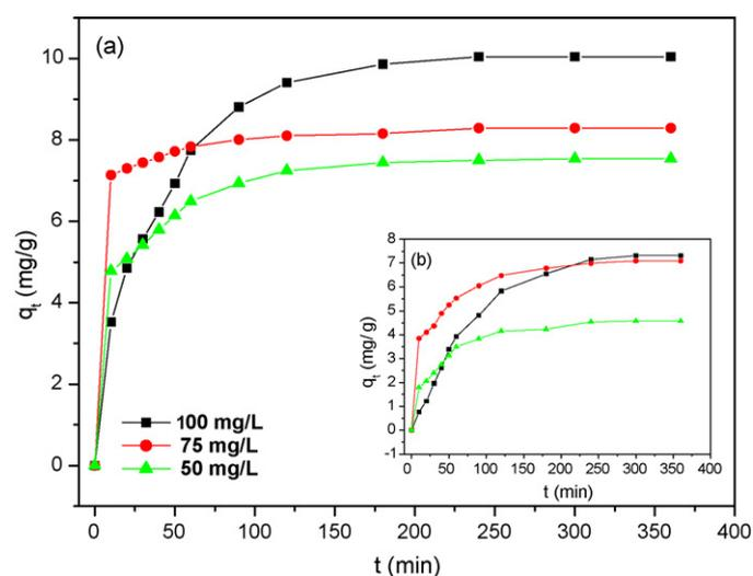
Fig. 6. Time-dependent adsorption of  $\text{Ni}^{2+}$  onto (a) Na-MMT and (b) A-MMT ( $\text{Ni}^{2+}$  concentration, 100 mg/L; adsorbent dose, 6 g/L; pH,  $6.5 \pm 0.1$ ; temperature  $25 \pm 0.1$  °C; 200 rpm).
