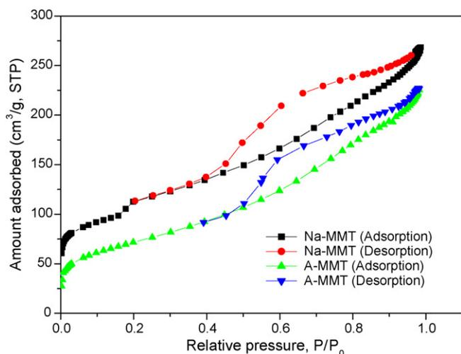
**Fig. 3.** Nitrogen adsorption/desorption isotherms on Na-MMT and A-MMT at 77 K.
