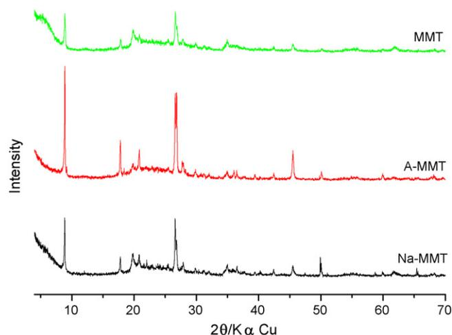
Fig. 1. XRD study of montmorillonites.
