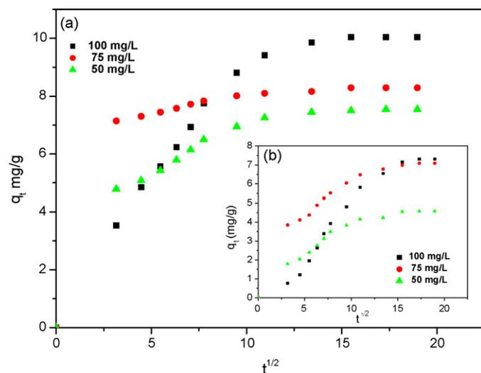
**Fig. 7.** Webber–Morris plots for adsorption of Ni<sup>2+</sup> onto (a) Na-MMT and (b) A-MMT (adsorbent dose, 6 g/L; pH, 6.5 ± 0.1; reaction time, 300 min; temperature 25 ± 0.1 °C; 200 rpm).
